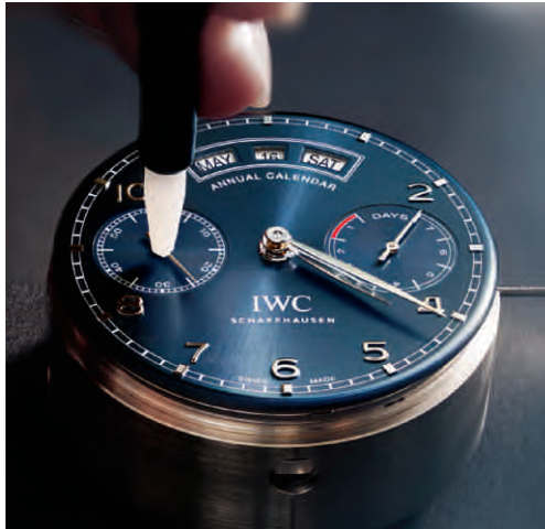
Once the test and function controls have been successfully completed, the dial and the hands are assembled
