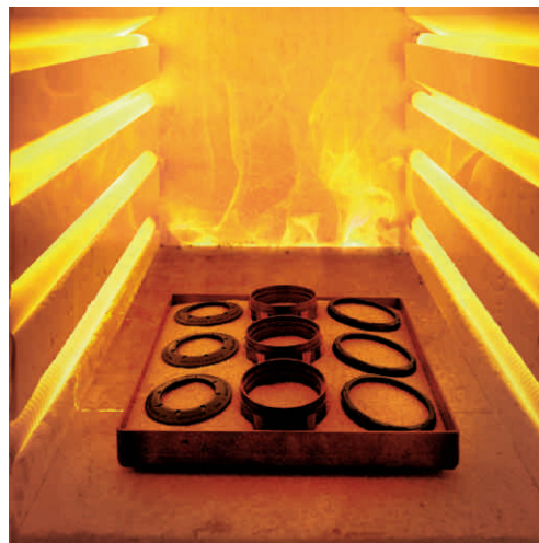
During the sintering process in the oven, the case components take on the striking matte black colour that characterizes Ceratanium®
